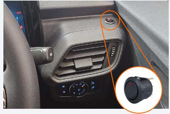
The Privacy Button is mounted on the driver's side of the dashboard, adjacent to the air vent.
